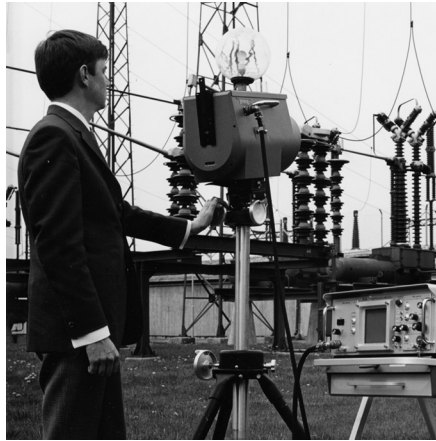
Figure 37.2 1969: Thermovision Model 661. The camera weighed approximately 25 kg (55 lb.), the oscilloscope 20 kg (44 lb.), and the tripod 15 kg (33 lb.). The operator also needed a 220 VAC generator set, and a 10 L (2.6 US gallon) jar with liquid nitrogen. To the left of the oscilloscope the Polaroid attachment (6 kg (13 lb.)) can be seen.
