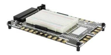
exhi:bit is a prototyping and development system for the BBC micro:bit that allows Makers or students to go seamlessly from a prototype to a finished, more permanent project.
