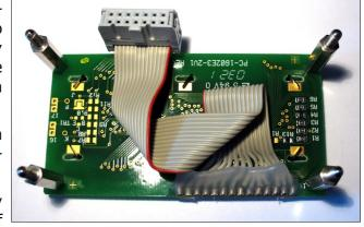
course, you will have to connect your own cable to the display unit (by soldering). Attention **must** be paid to the correct pin assignment!
