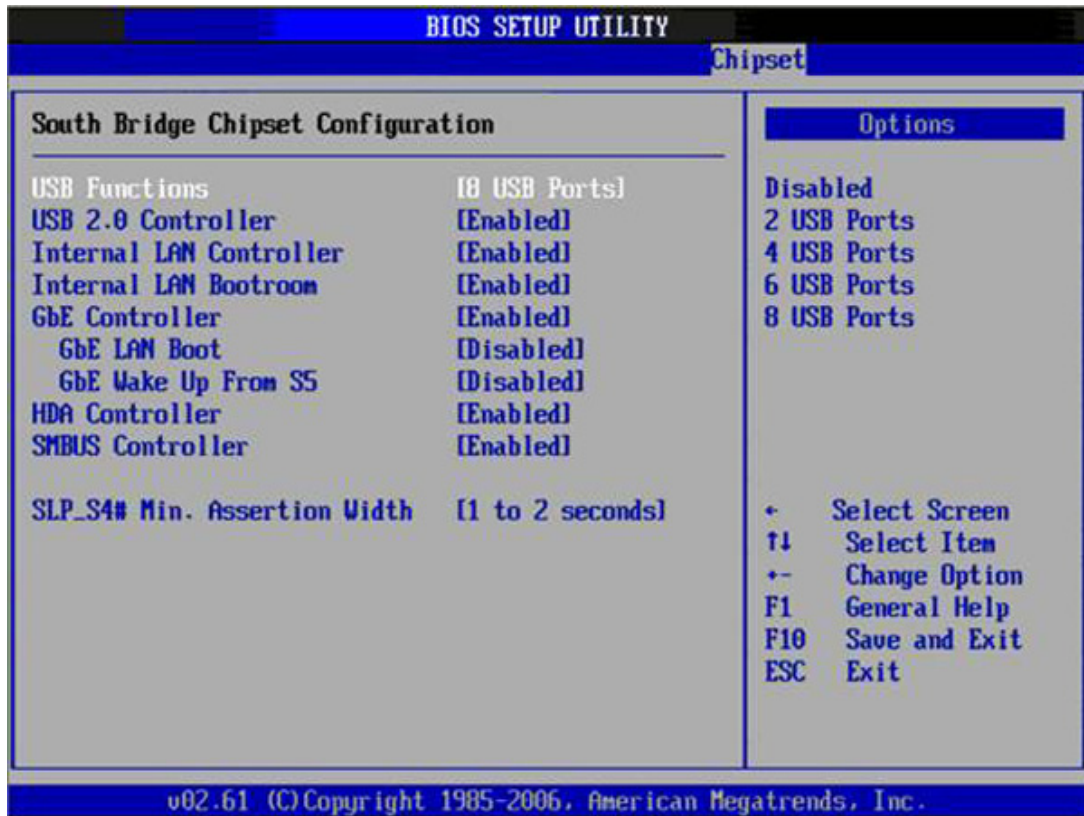
Figure 3.26 South Bridge Configuration
