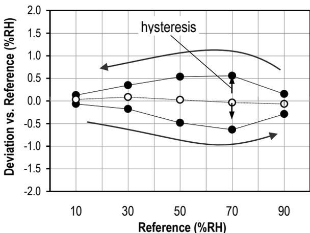
**Figure 2** Example for hysteresis measurement. A path from dry to humid and one from humid to dry is measured – full dots on graph. Dwell time at each log point is 30 minutes. Open dots determine mean values – representing calibration accuracy.
