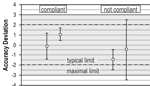
**Figure 3** Examples for accuracy distributions complying (left side) or not complying (right side) with the specified accuracy range. Open dots represent average values. Error bars denote 2k range and must stay within typical limits.
