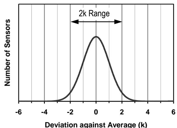
**Figure 1** Distribution of sensor deviation around average.  $2k$  range must fit into typical specification band. The coverage factor  $k$  is equivalent to standard deviation  $\sigma$  in case of normal distribution.
